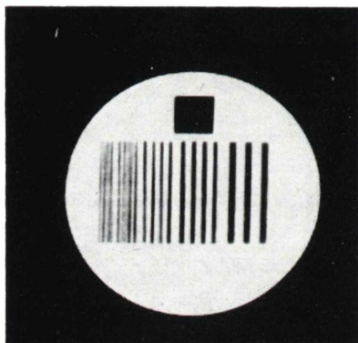
Fig. 1 Slit phantom image. 256 SR (500), Their widths of each slits are 1.5 mm, 2 mm, 3 mm, 4 mm and 5 mm from thin to thick slits, and 2 mm slits are apparently clear.
