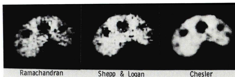
Fig. 2 Transaxial images of the phantom reconstructed by using various filters. The Chesler's filter was considered to be suitable for clinical use.
