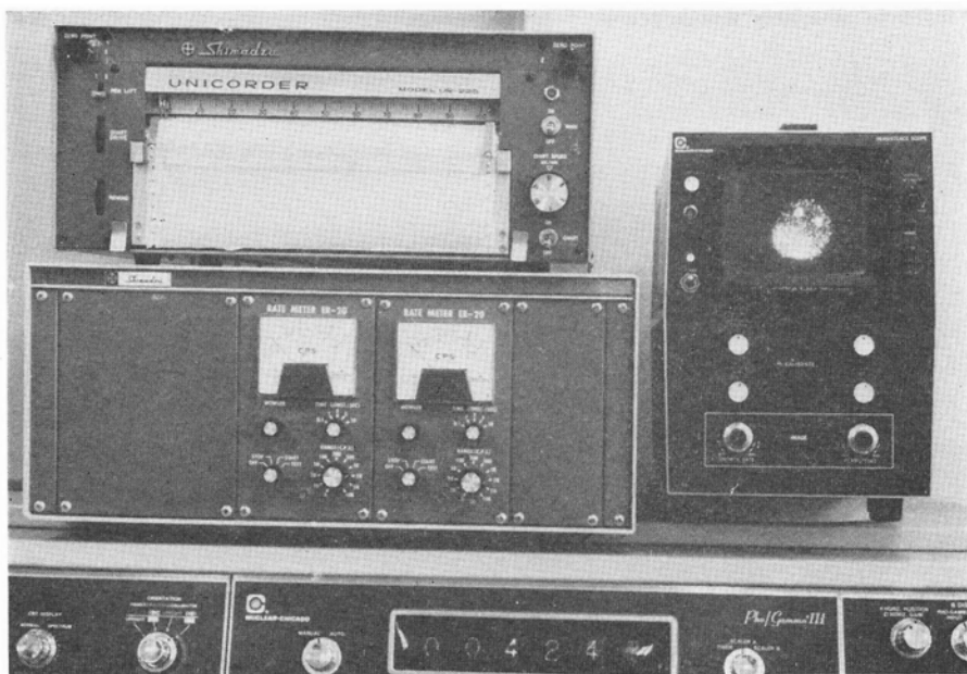
Fig. 1. Data of the Data-store play-back system are reprojected on the Persistence scope. There, areas of same shape and same size are settled for both abnormal and normal portion, and time histograms are obtained by the Rate meter. Thus, successive dynamic change of RI within the abnormal portion is observed.
