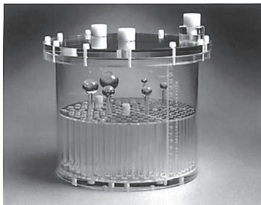
Fig. 1 Jaszczak phantom with cold rod inserts, hot and cold spheres.
