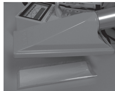
Fig. 1 A PSSM (TCS-316H, Hitachi Aloka Medical, Ltd.) was used to measure for 10 minutes the radioactivity of a 50 \times 150\text{-mm} piece of polyethylene filter paper that had absorbed 2\text{ ml} of a solution containing a ^{89}\text{Sr} concentration of 14\text{ Bq/ml} .
