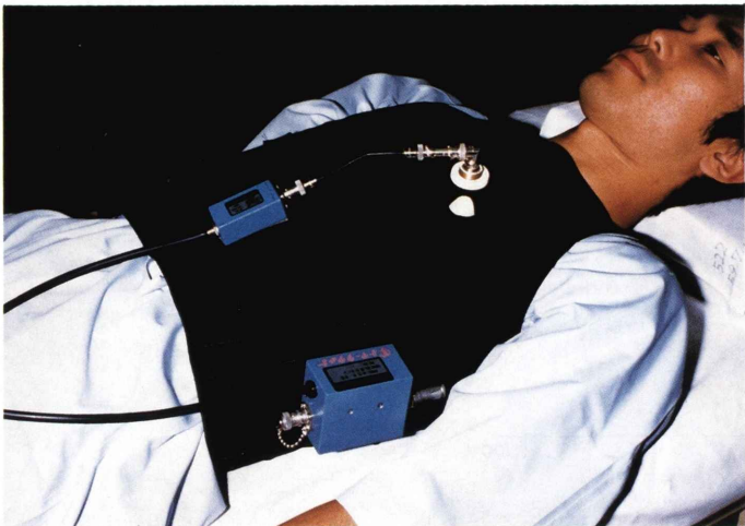
Fig. 13 Our new vest-system for the attachment of the probe to the chest.
