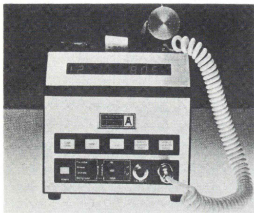
Fig. 1 If-scan (Crystal: 38 mm diameter \times 2 mm thick, Analyzer: ^{125}\text{I} -window).
