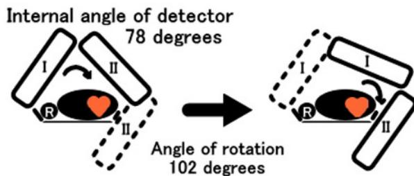
**Fig. 1** Data collection for 180 degrees with a two-detector system. Imaging is not affected even when the right arm is not raised.
