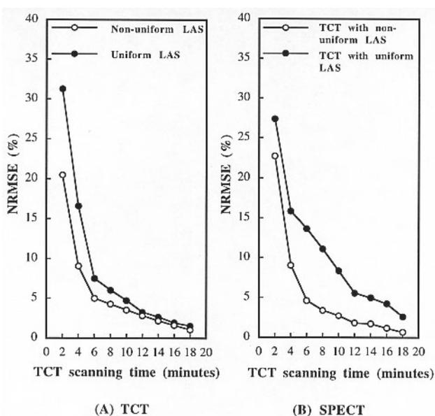
**Fig. 5** Comparison of normalized root mean square error (NRMSE) between the non-uniform LAS and the uniform LAS on TCT images (A) and SPECT images (B) with different scanning times. By means of the non-uniform LAS, an acceptable NRMSE of less than 5% in the SPECT image was achieved with the 6 minutes-TCT scanning time.
