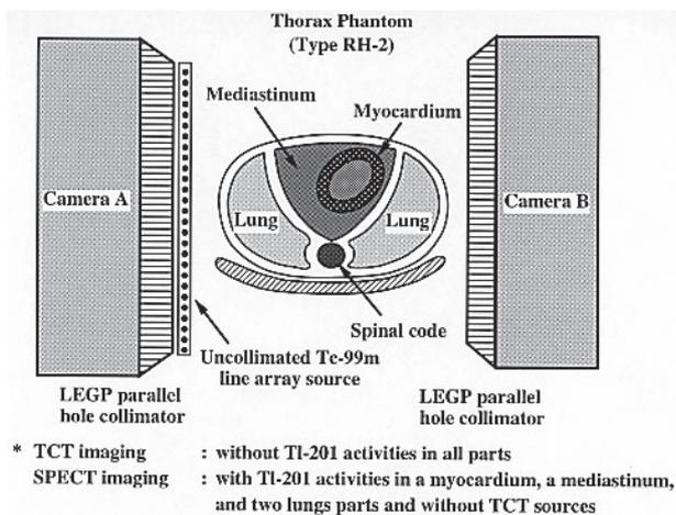
Fig. 2 TCT and SPECT imaging using a thorax phantom.
