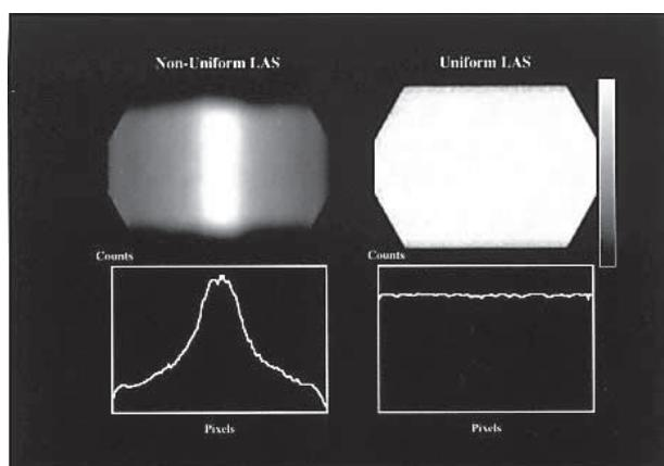
Fig. 3 Comparison between the non-uniform LAS and the uniform LAS on planar images (blank data) and count profile curves. Due to the blurred spatial resolution, the blank image with the uniform LAS had a uniform count distribution at the whole field of view, but that with the non-uniform LAS gave a smooth mountain shape with high count rates at the center and low count rates at both sides.
