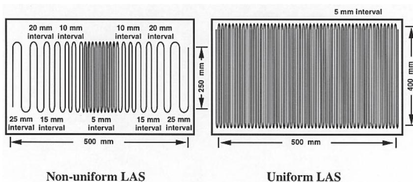
Fig. 1 Uncollimated Tc-99m line array source configurations.
