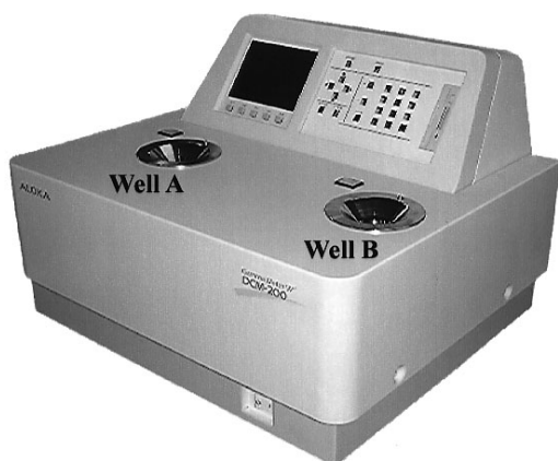
Fig. 1 Photograph of a double-well single-plastic scintillation counter (DCM-200, Aloka Co., Tokyo, Japan). Well A is for a sample-tube with a low radioactivity and well B is for an injection syringe with high radioactivity.
