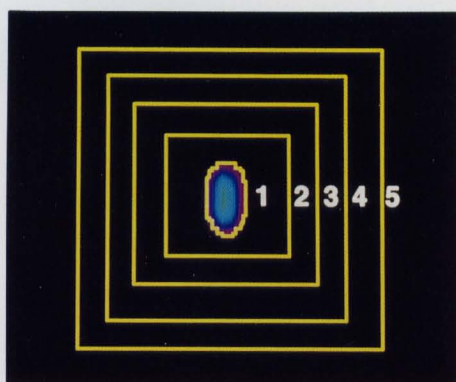
Fig. 3 ROI positions around the line source. ROI1-line source area (256 pixels), ROI2-30 \times 30 pixels, ROI3-50 \times 50 pixels, ROI4-70 \times 70 pixels, ROI5-90 \times 90 pixels
